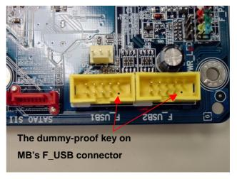
3. Please connect the cables of bracket to the proper connector with the same color. Purple/gray connector is for F2\_1394 (pruple) /F1\_1394 (gray) connector; yellow connector is for F1\_USB or F2\_USB connector.
